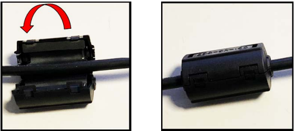
Example of how to mount a ferrite
