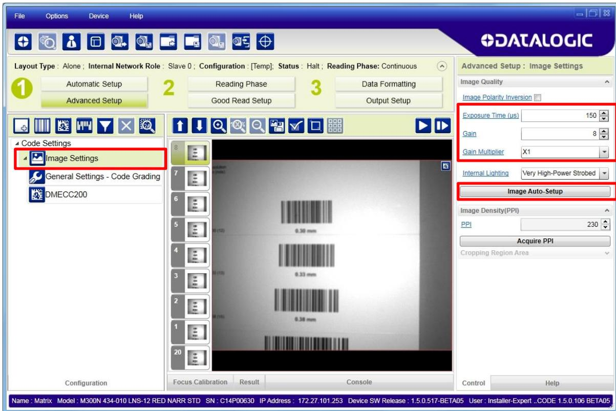
4. Select the Static or Dynamic Self-Tuning option; Start the Image Auto Setup and Apply to the Image Settings.
