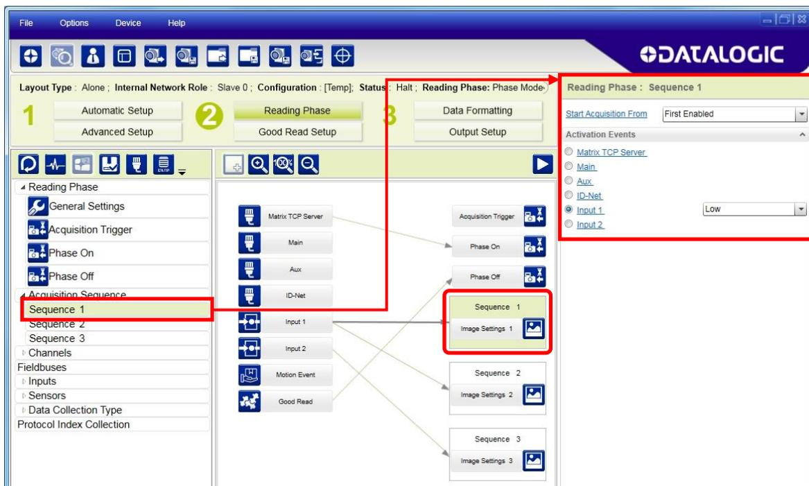
Alternatively a hybrid configuration can be made where more than one **Image Setting** can be grouped into an Acquisition Sequence by dragging it into the desired Sequence box. Select the empty Sequence box and delete it with the delete key.
