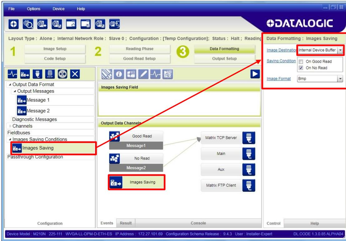
To download the saved images, the device must be in offline mode. Through the Device menu>RAM Image Buffer you can access the **Image Buffer Management** window.
