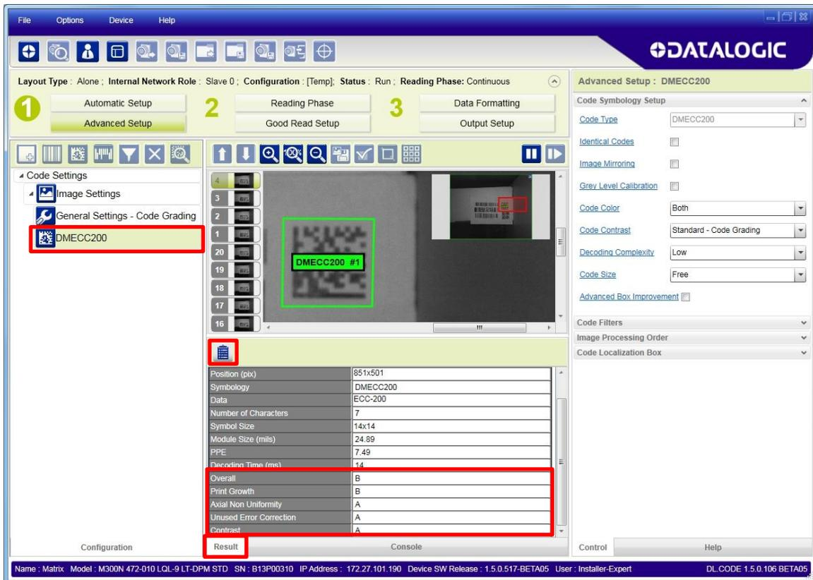
The output message can also be defined to include the scan grade parameters.
