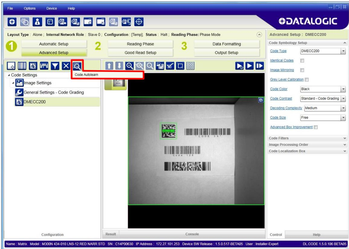
The Autolearn region (equal to the FoV) is shown in grey. You can reduce and/or move the search area by dragging the borders or the center of the area with the mouse.
