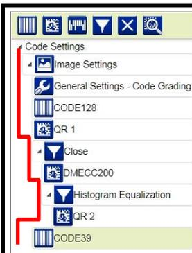
Since the visual effects in the image area are overlapped, you should not use this as a reference to determine how and where Image Filters are applied. You must read Image Filter application from the Tree structure in the configuration parameter tree area. The example in the figure to the left shows:
