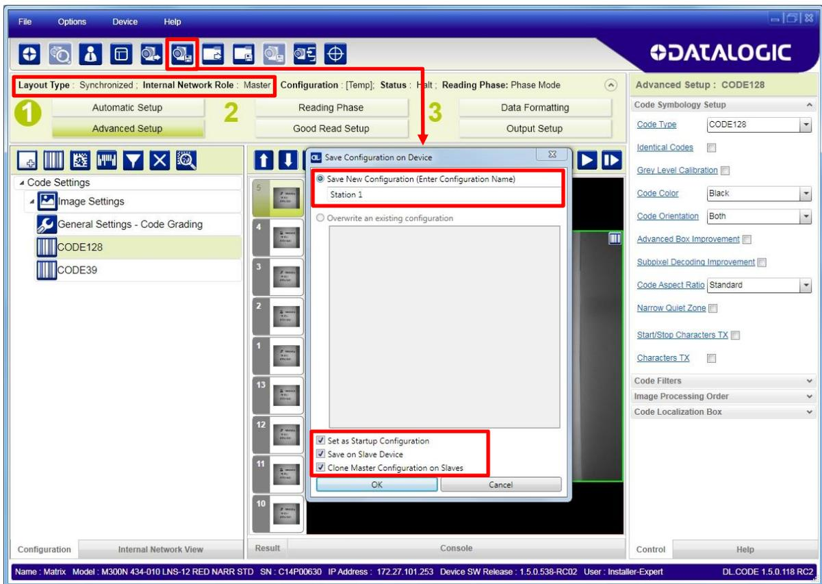
Figure 12 – Saving Synchronized Phase Mode Configuration to Master
