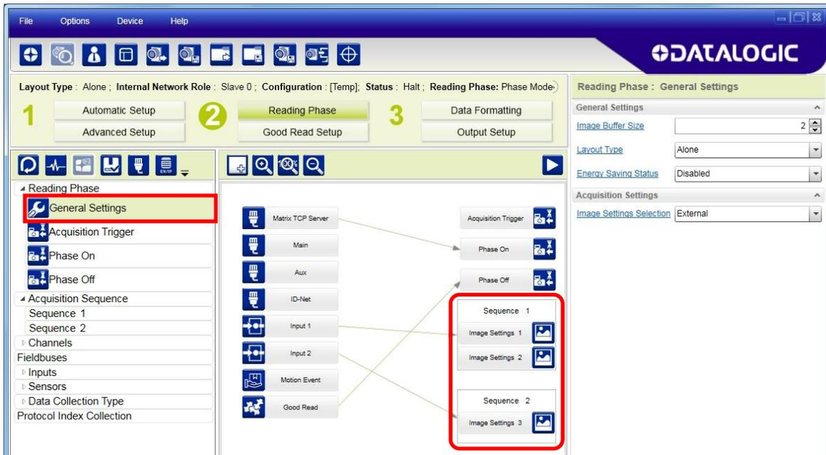
Each **Acquisition Sequence** can be activated exclusively by a single event, either through a string from an available communication channel or by a digital input.
