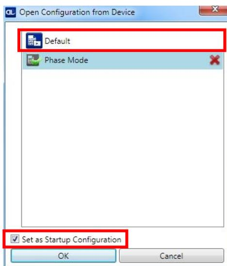
The same action can be performed from the Device menu >Backup/Restore > Restore Defaults > **Restore Default Startup Configuration**. The Default Configuration will be set to run at startup and the reader will be reset.
