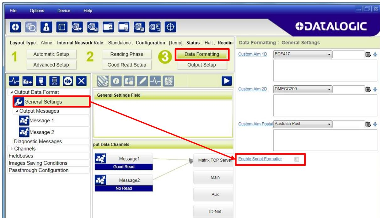
The Script Formatter will now replace the Output Messages branch. It is complete with several editing tool icons to facilitate scripting within the DL.CODE GUI.
