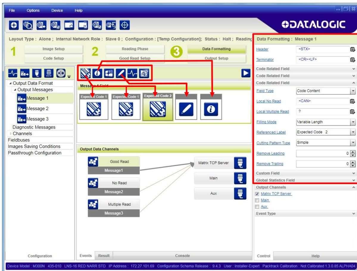
The DMECC200, QR Code and Code128 types are enabled and present in the Code Combination with the following logical combination:
