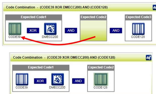
To create a logical AND condition from a logical XOR, create a new Expected Code box using the
