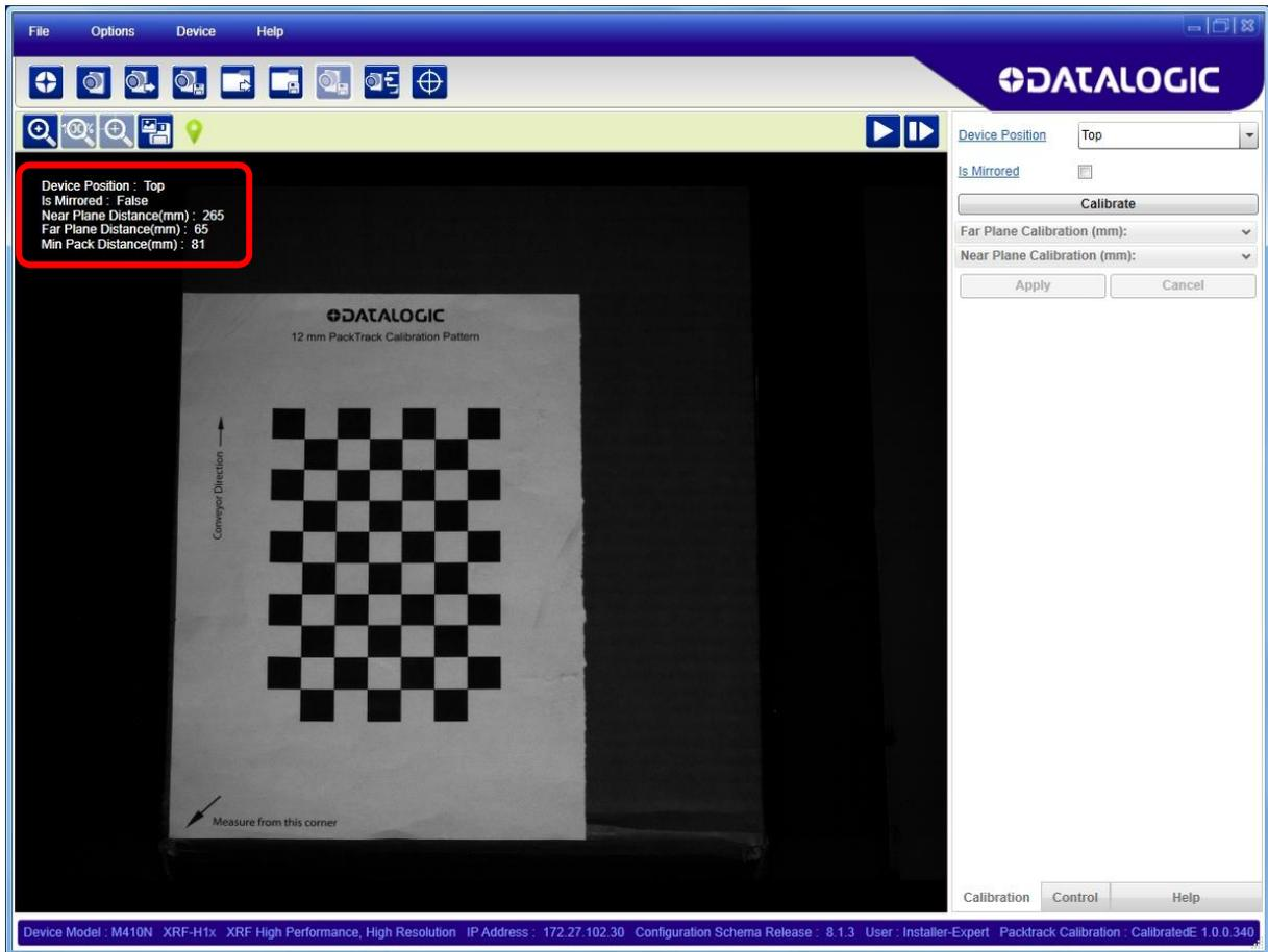
The calibration also advises the minimum distance between packs (Min Pack Distance), for which correct code to pack assignment can be guaranteed.
