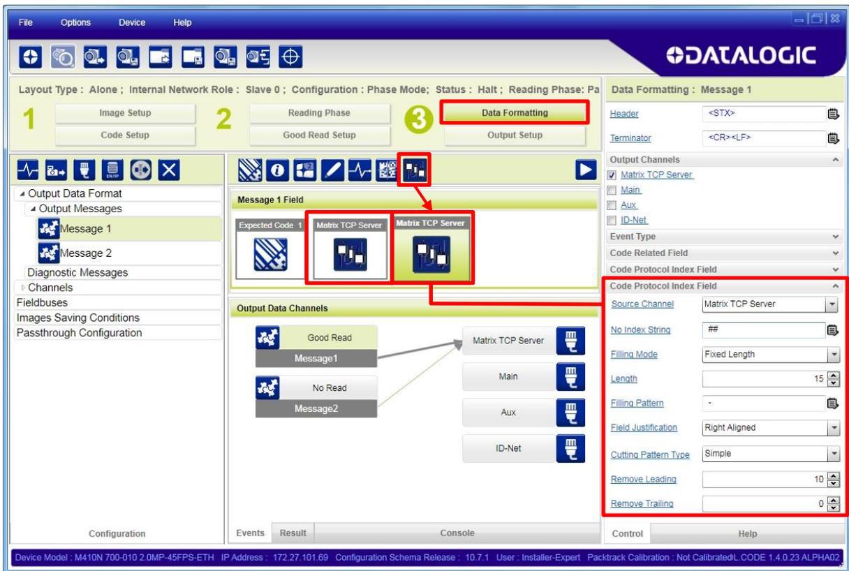
For further details on the Protocol Index Message, see the parameter descriptions in the DL.CODE Help On Line Protocol Index page.
