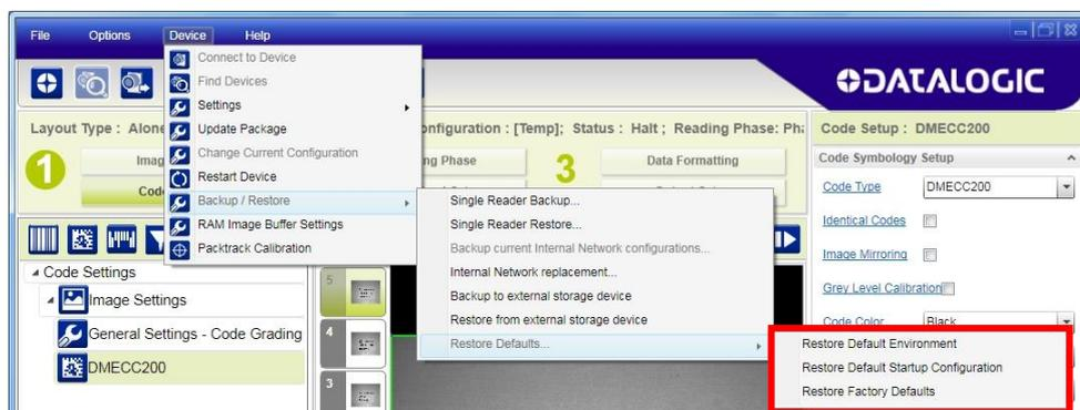
Any previously saved configurations on the device will remain in memory, but the Default configuration is set as the startup configuration.
