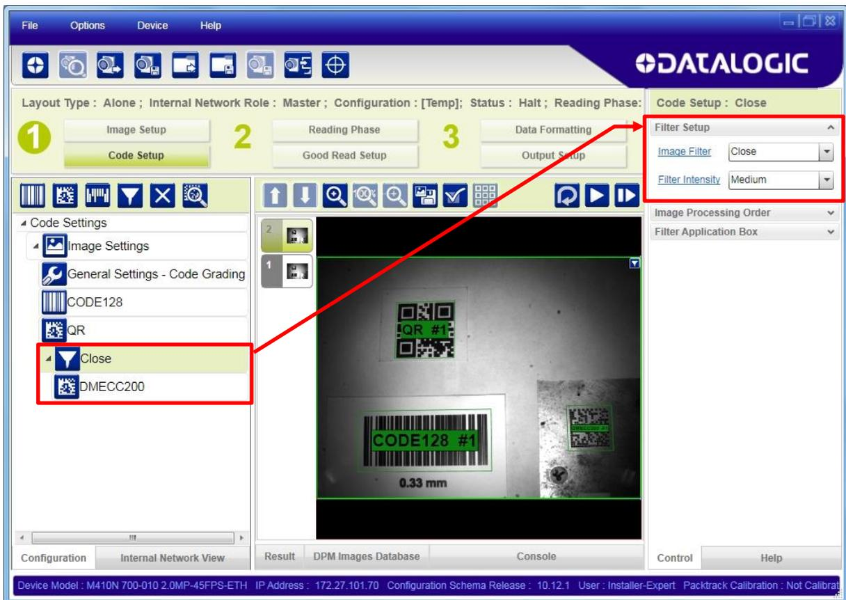
The Data Matrix DPM code is now successfully decoded; Code Localization box as well as code bounding box are colored green.
