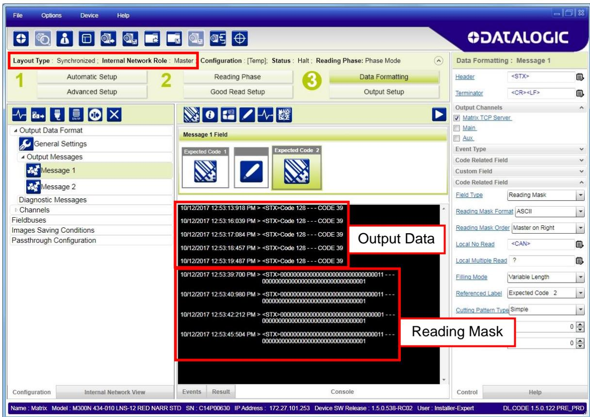
The Reading Mask shows which device reads which Expected Code. The mask is composed of a fixed 32-character string (0=No Read or 1=Read) representing the 32 possible readers in an ID-NET network. By default the Master is the last character in the string (**Master on Right**) but this can be changed. The Slaves are shown adjacent to the Master in order (1 to 31), by default from right to left.
