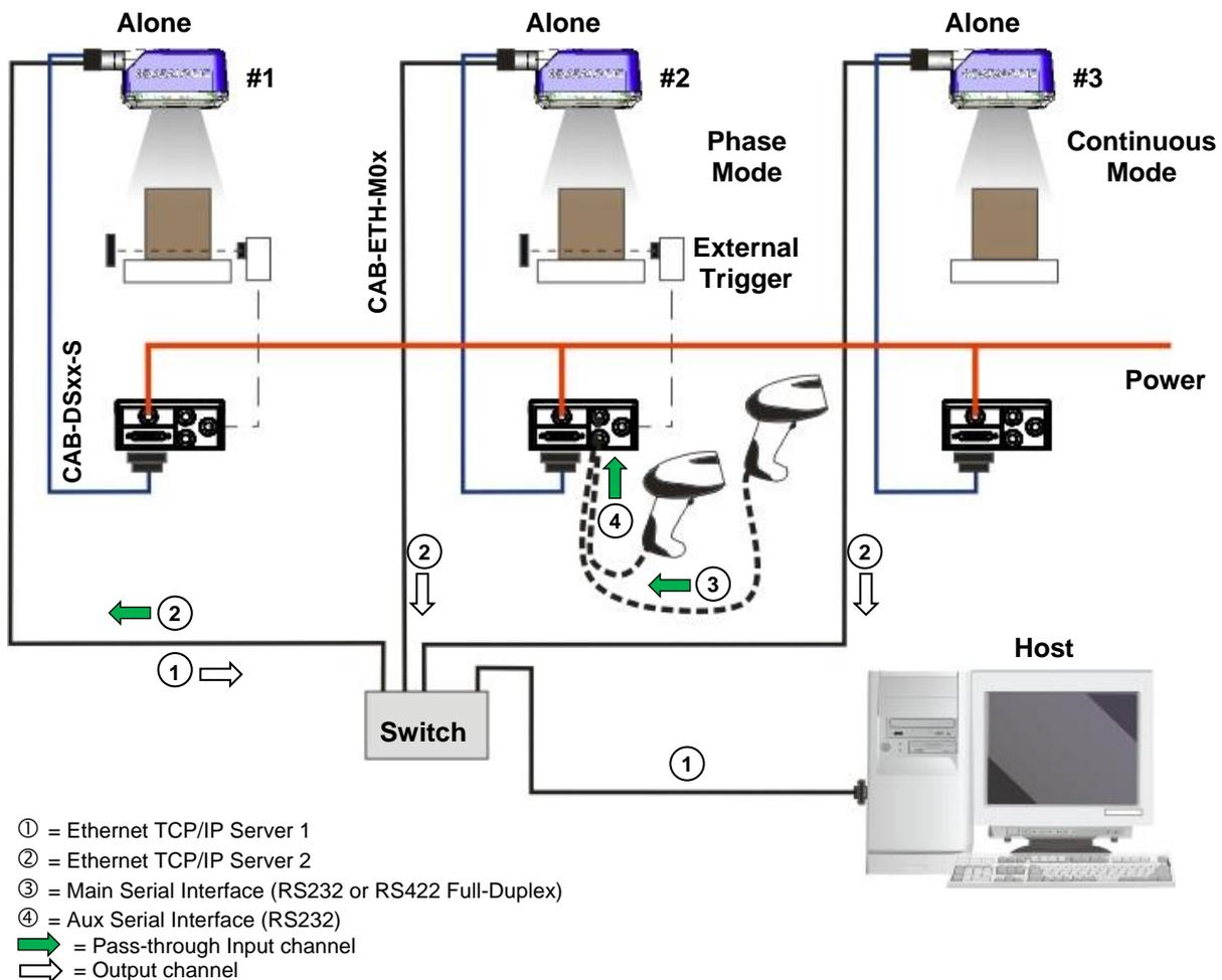
Figure 8 – Example Pass-through Layout
