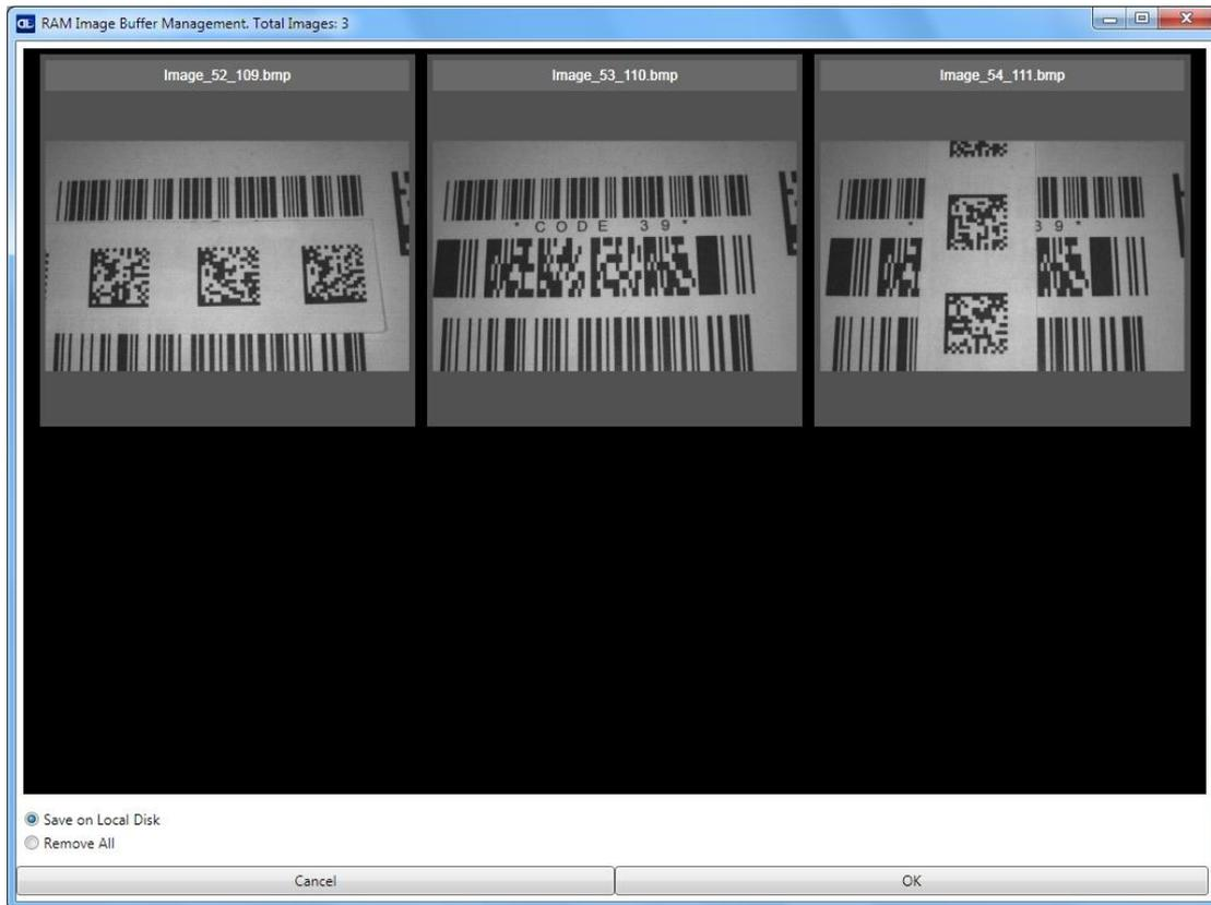
Upon opening this window, the images in the Device Image Buffer (RAM) are transferred to the DL.CODE Device Image Buffer Management window and the images are deleted from the device RAM.
