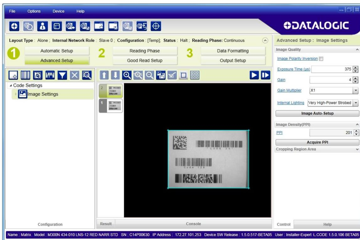
You can also set the cropped image size and position through the Cropping Region Area group of parameters; size = **Width** and **Height**, position = **Left**, **Top** (x,y) coordinates.
