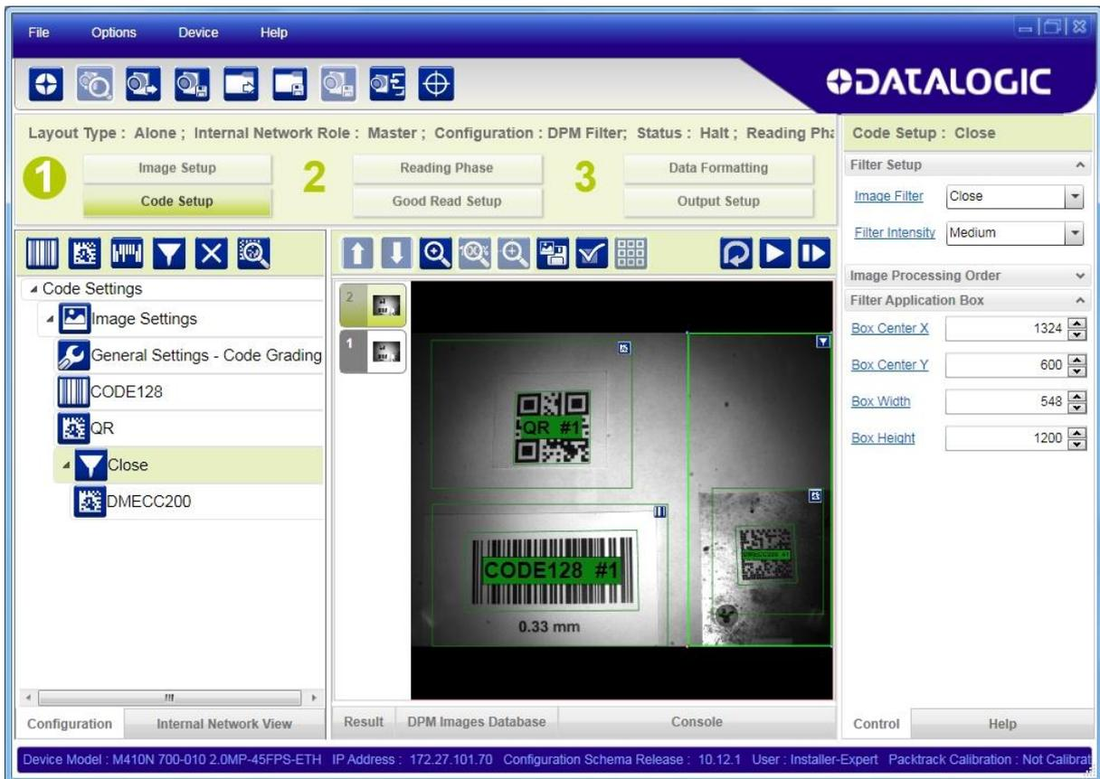
The following steps are taken to apply the Close filter to Example 2:
