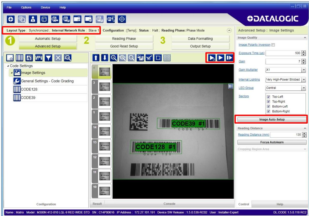
Verify the focus and decoding with the capture image
