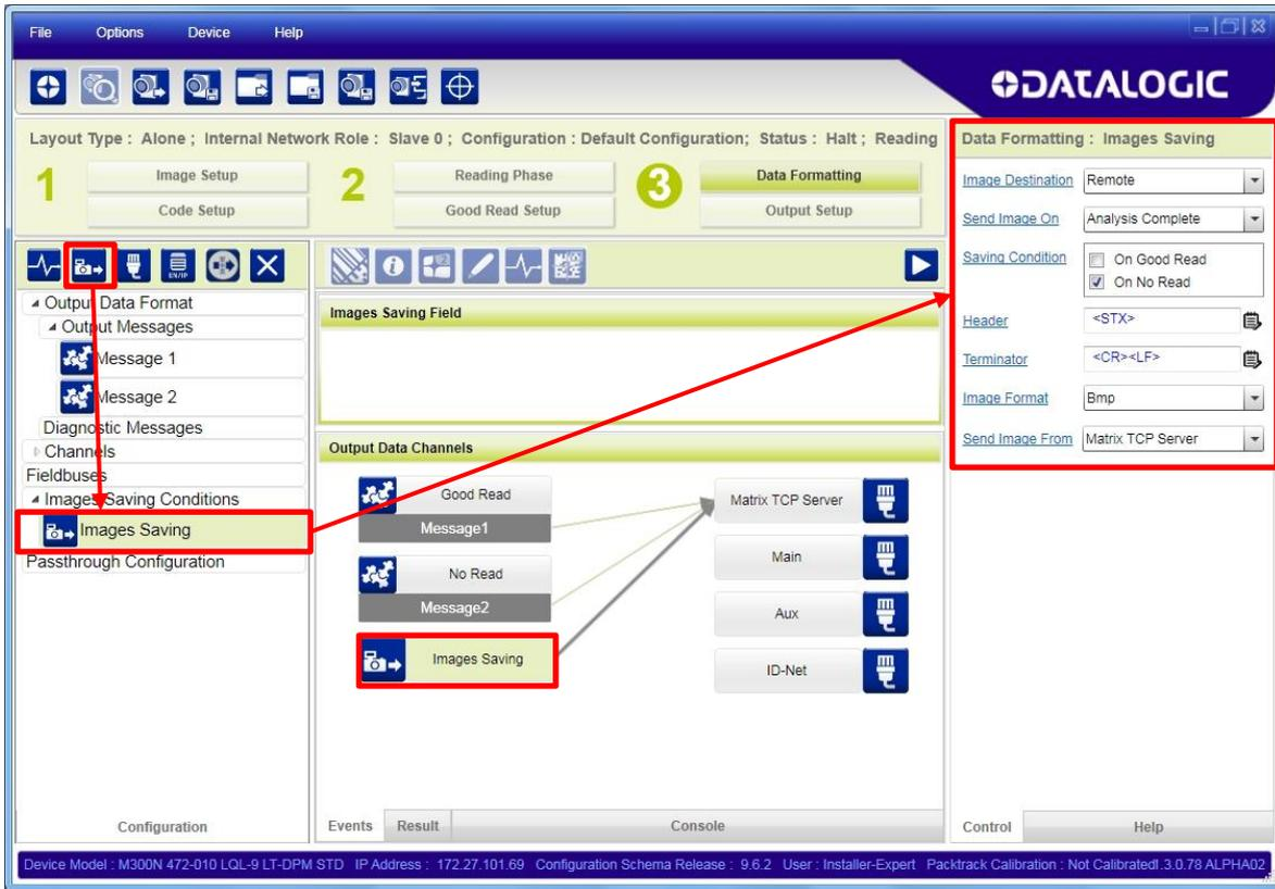
When selecting a Remote **Image Destination**, the default value is **Send Image From** Matrix TCP Server (on-board Ethernet) channel to an external TCP Client. If desired, a different dedicated Matrix channel can be added for image transfer.
