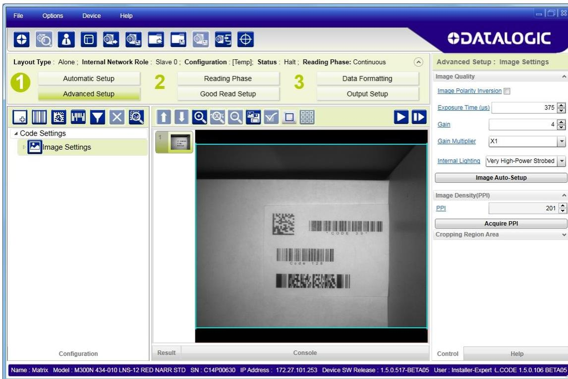
By dragging the edges with the mouse (resizing) you can crop the image to a specific location where codes are present. The numbers in the blue boxes refer to pixel references.
