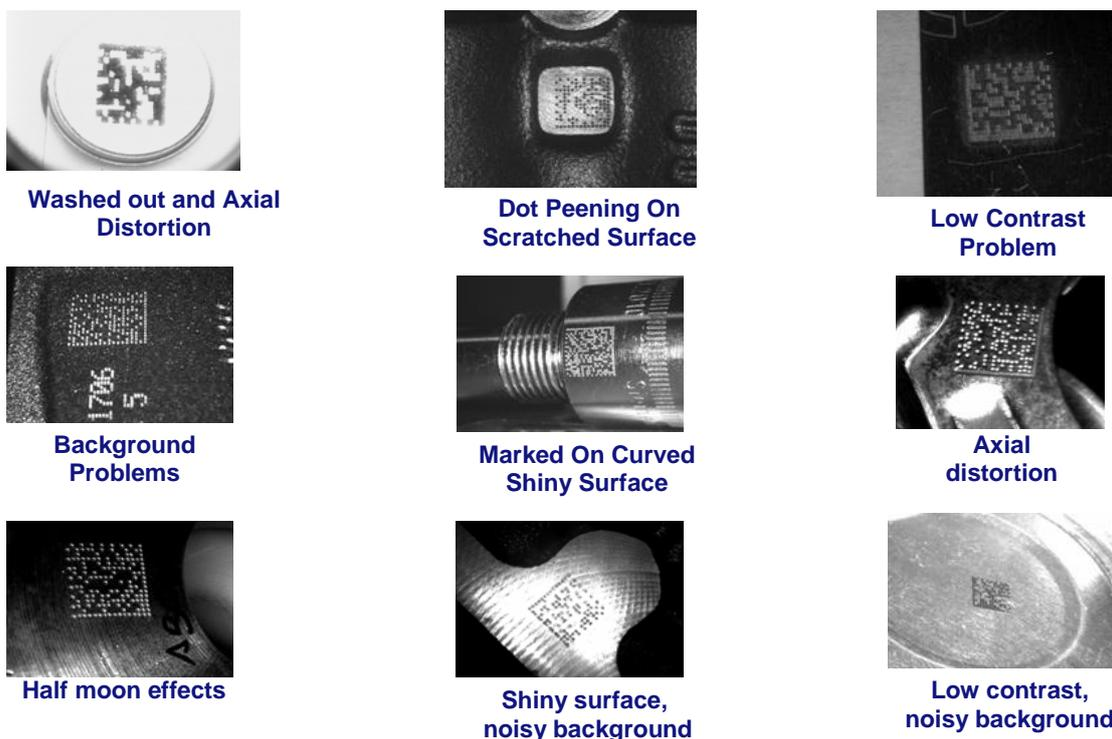
Figure 7 – Problematic Direct Part Marking Examples
