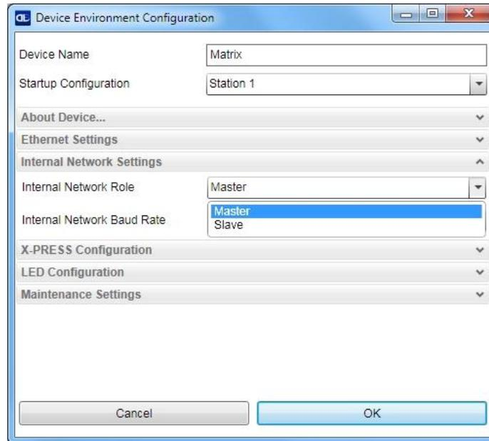
Wait for the device to reset. It may be necessary to wait several seconds and then perform a Discovery to refresh the device list area. You should now see the Master device with its relative icon.
