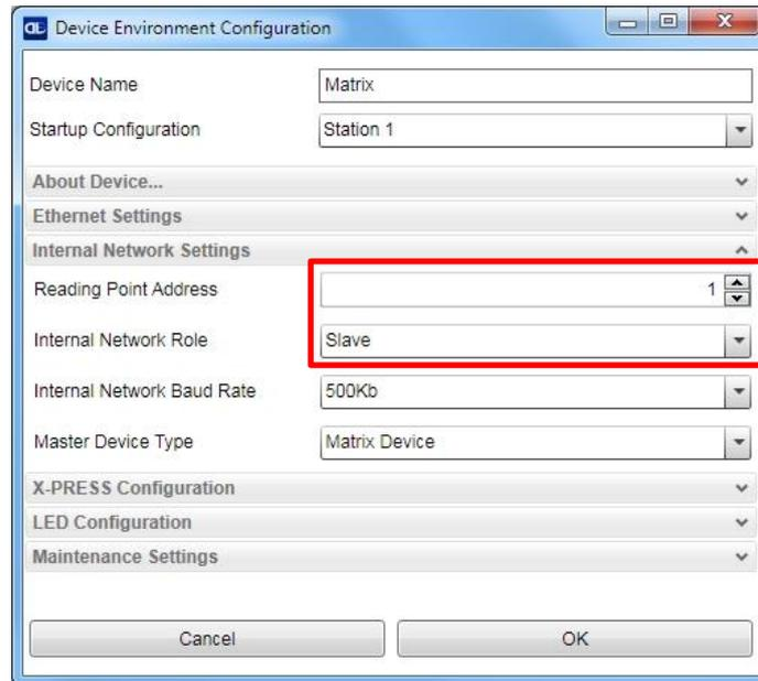
Complete the Slave configuration and save it to the device.
