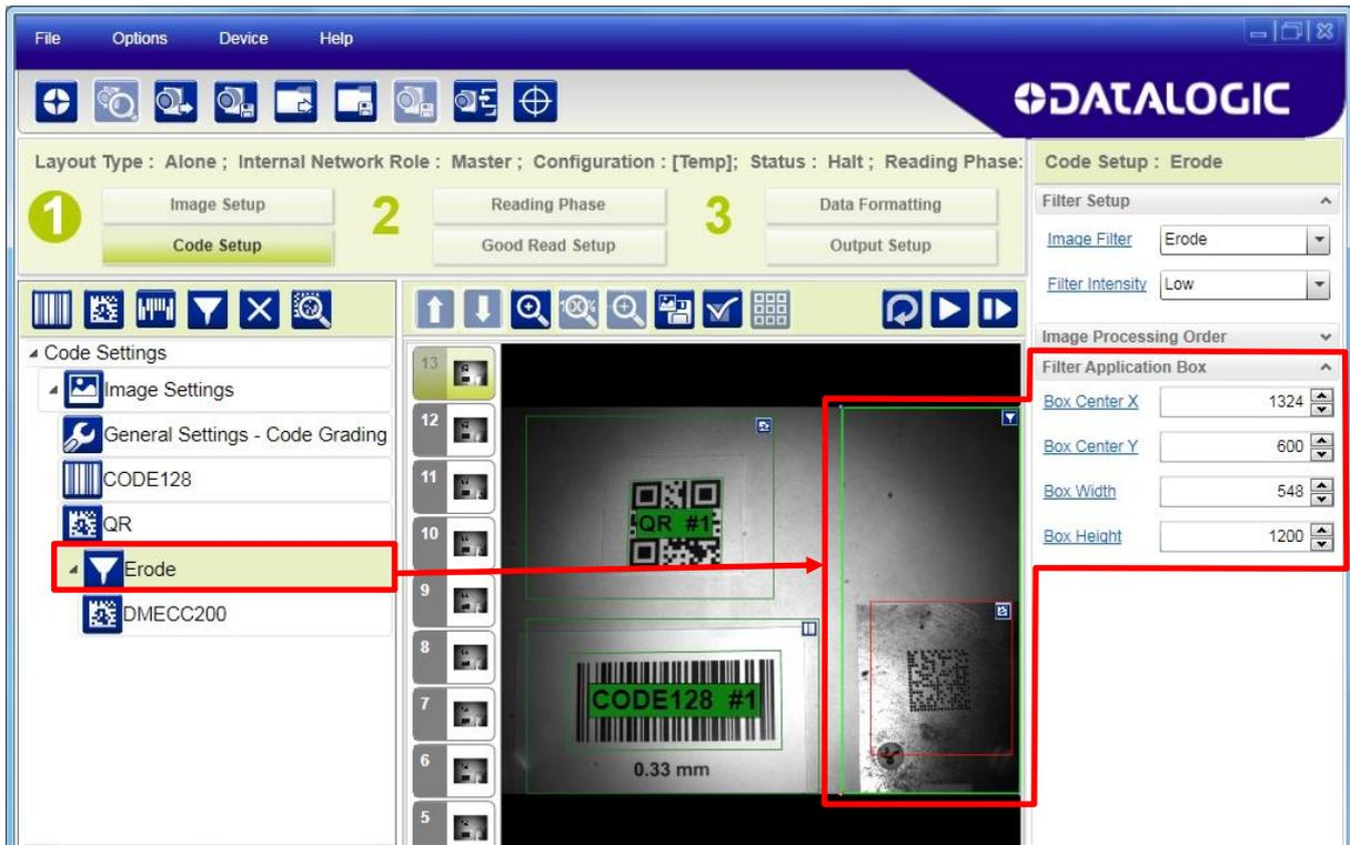
5. Select the desired Image Filter Type and Intensity for correct decoding.
