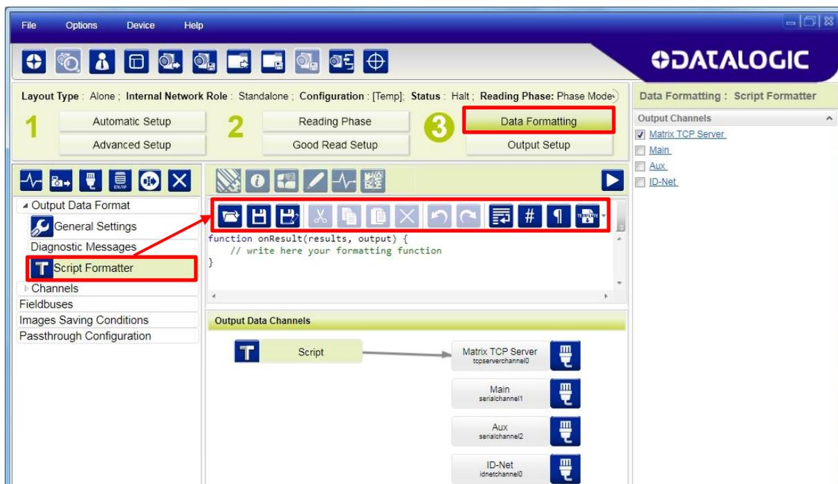
Script Formatter is based on an embedded JavaScript engine. For DL.CODE version 1.5.0 and later, the embedded JavaScript engine conforms to ECMAScript 5.0/5.1 Language Specification.
