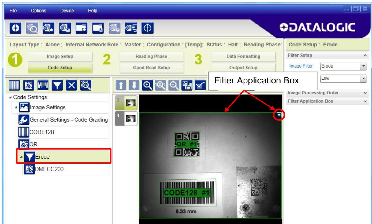
3. Select the desired Image Filter Type and Intensity for correct decoding.
