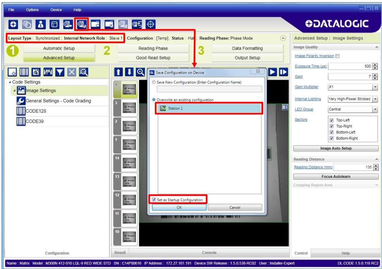
Figure 13 – Saving Synchronized Phase Mode Configuration to Slave
