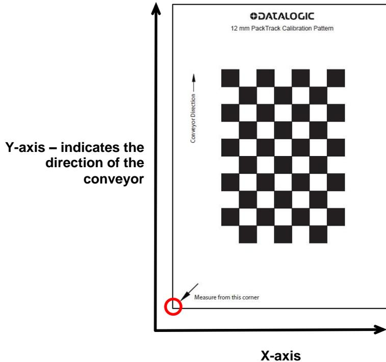
During the calibration process the user has to input the coordinates measured from the System Reference Point to the **lower left corner of the Calibration Pattern** indicated by the red circle.
