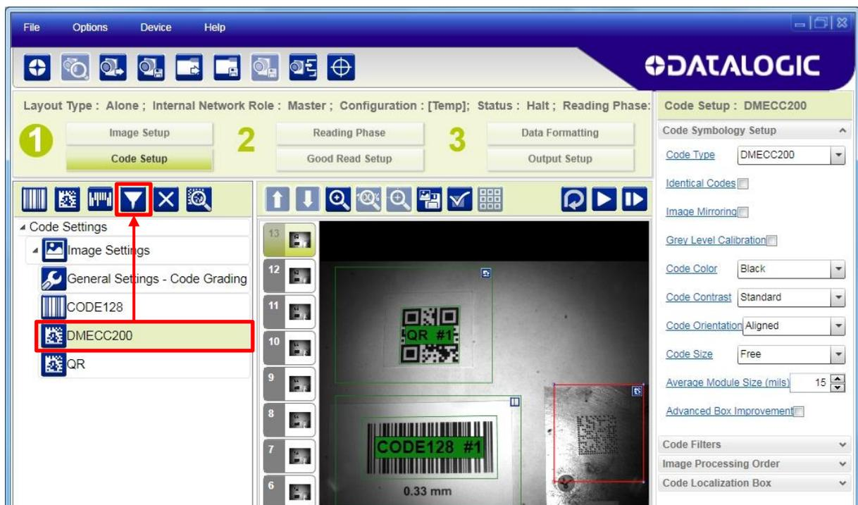
4. Resize and position the filter application box (dragging its borders with the mouse or editing the Filter Application Box parameters) to the image area where the filter will be applied. The relative Code Localization box must fit inside its Filter Application box.
