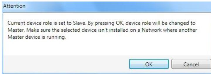
Click OK. The Net Autoset feature automatically starts to find Slave devices connected to the ID-NET network of the Master.
