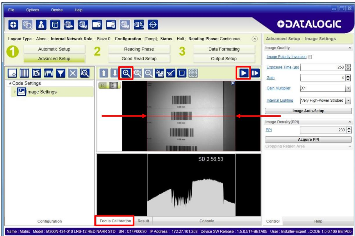
The red line in the image panel above the oscilloscope must pass through the code. You can click and drag the red line vertically to reposition it over the code.
