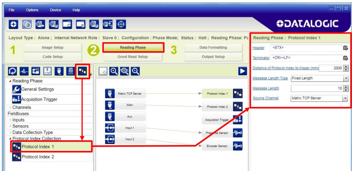
*Header* and *Terminator* strings must be configured whenever a new Protocol Index object is added to a configuration. Either *Header* or *Terminator* can be blank but not both at the same time.
