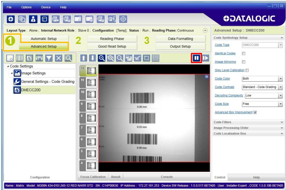
3. Click the Image Settings branch and then click the Image Auto-Setup button to automatically acquire the best exposure time and gain values.
