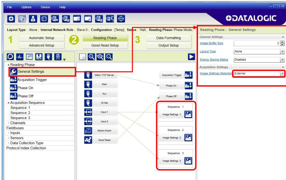
Each **Acquisition Sequence** can be activated exclusively by a single event, either through a string from an available communication channel or by a digital input.
