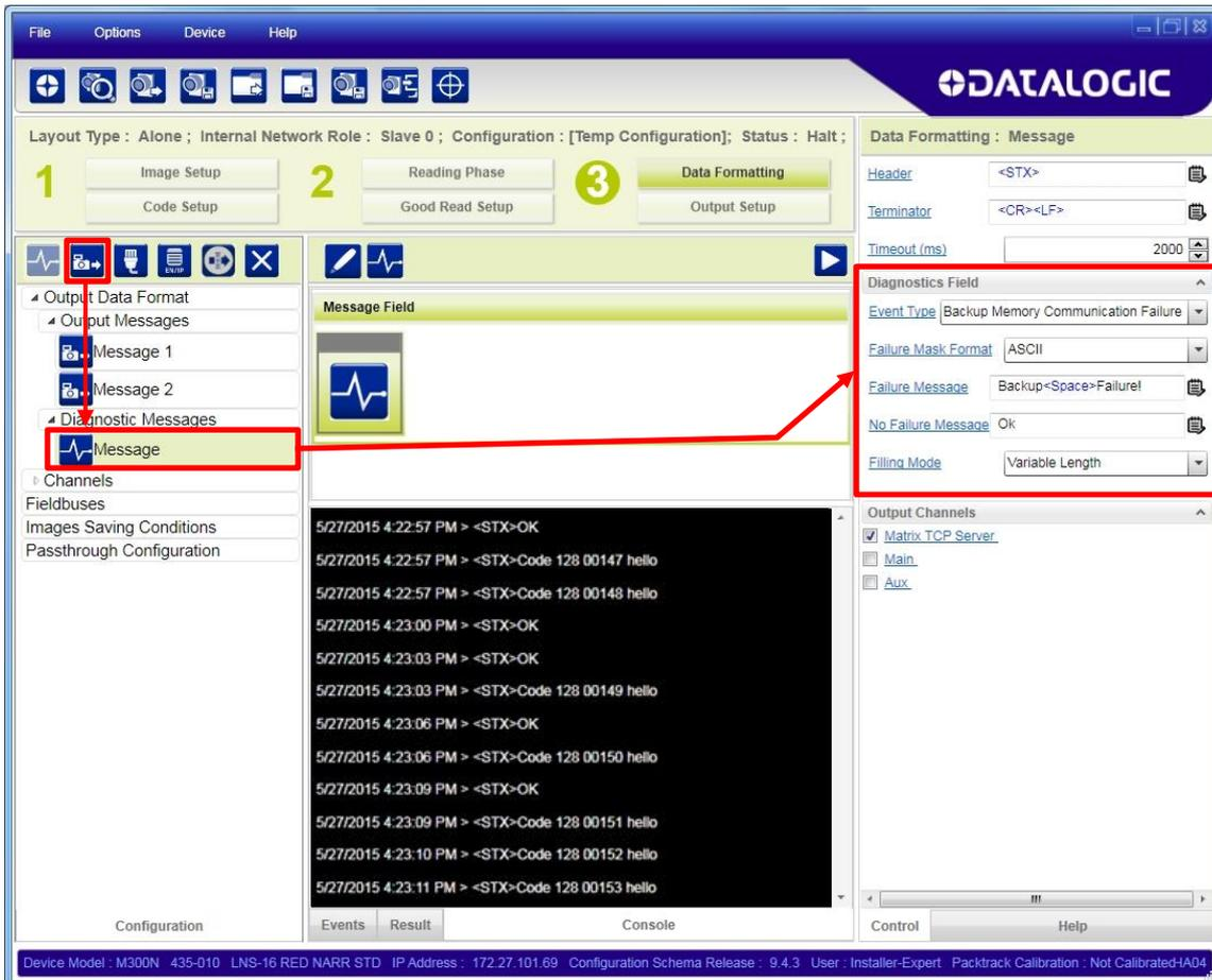
Typically only the Failure string is defined to avoid unnecessary message traffic.
