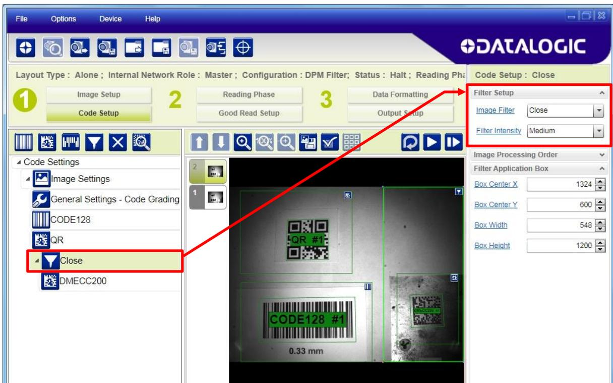
The Data Matrix DPM code is now successfully decoded only within the expected position; Code Localization box as well as code bounding box are colored green.
