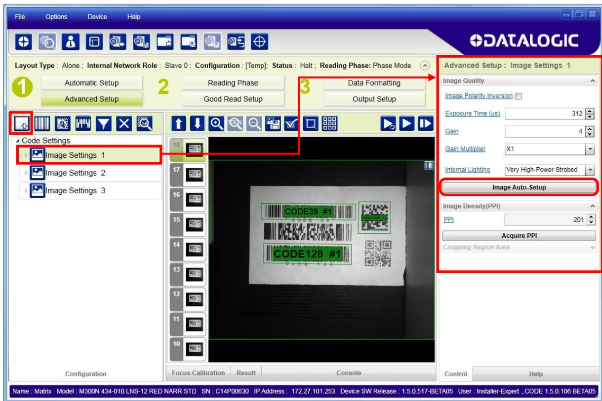
For each Image Setting condition start **Image Auto Setup**, select the Static or Dynamic Self-Tuning option; and Apply it.
