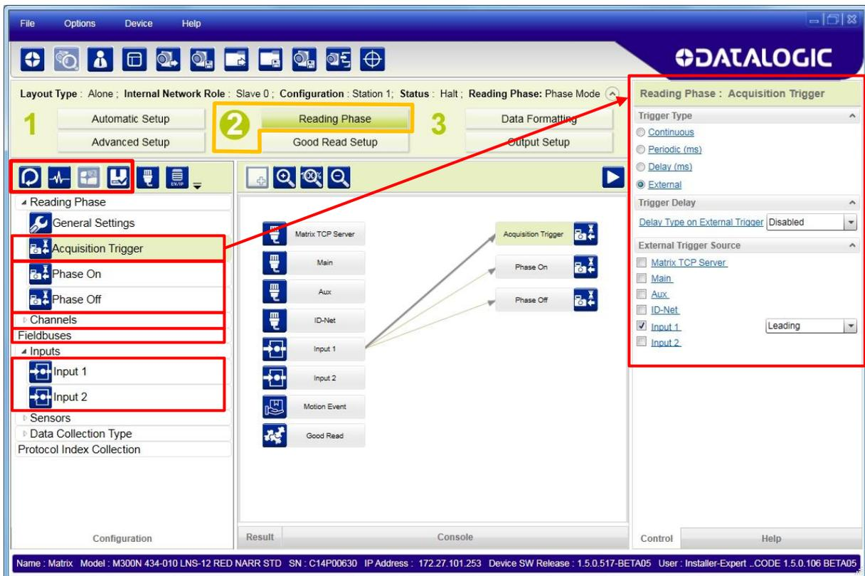
2. Configure the relative Operating Mode parameters from the Reading Phase parameters panel. Different groups will appear in the panel depending on the selected icons over the Configuration Parameters tree area.
