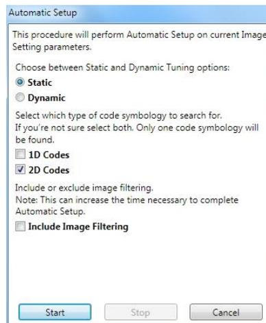
6. Select the correct reading conditions: Static or Dynamic Tuning, 1D or 2D code, Include Image Filtering (to find the best decoding condition).
