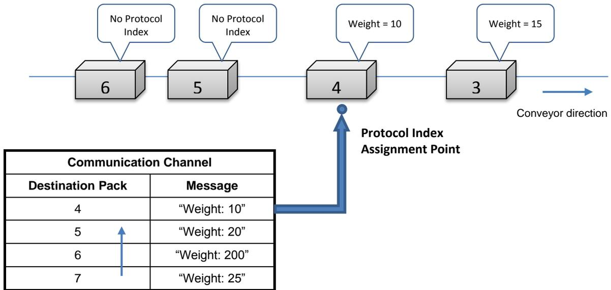
Protocol Index can be used either in Phase Mode (during the active reading phase) or in PackTrack operating mode (between the PS Offset and the Tx Line Distance).
