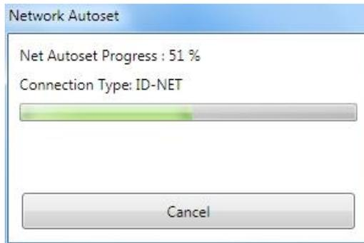
When finished, all the Slaves should have been correctly recognized. If not, verify all device connections and power and then repeat the operation by clicking on the Start Net Autoset button.
