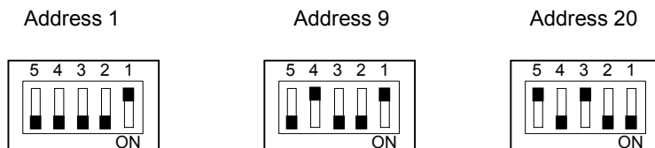
Figure 18 - DP1100 multidrop address selections
